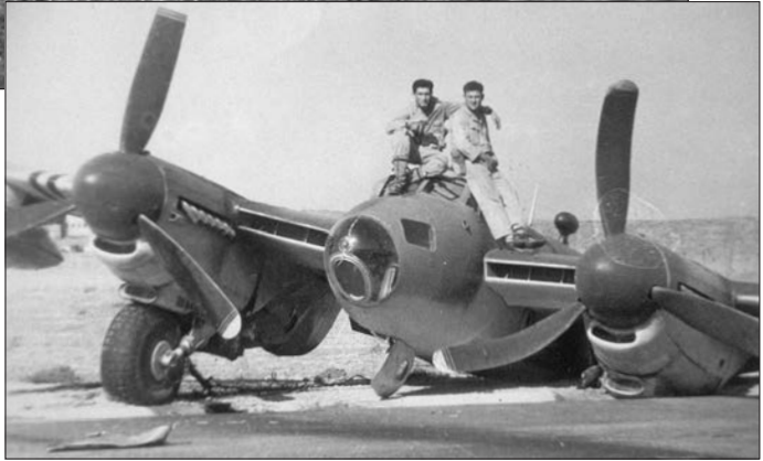
Aircraft 90 was one of the last three Mosquito planes to arrive in Israel in 1956. It is shown here after its right landing gear broke during landing on November 22, 1956. As seen in the image, the fuselage is damaged, and the aircraft was subsequently grounded. The markings from the 'Sinai Campaign' are visible on its wings and fuselage.
